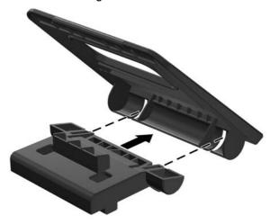
3. Slide the hooks at the top of the stand into the slots on the rear of the monitor panel (1) then snap the latches on the stand into the latch holes on the monitor (2).
